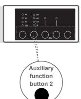
You can gradually decrease the washing water temperature between the maximum washing water temperature of the selected programme and cold washing \*\* selections by pressing temperature adjustment button.
